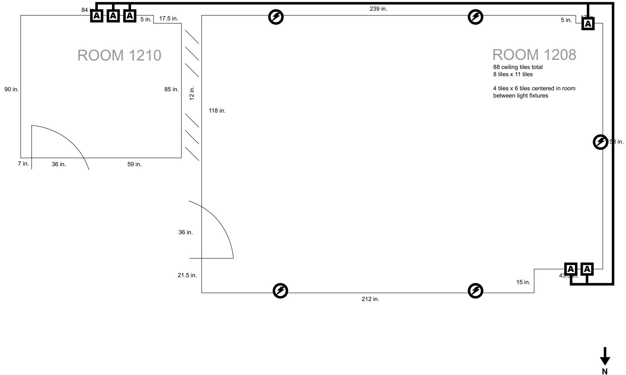
**Floor Plans:** Modular Audio Production Space : Wall plates for Audio and Electric including Audio Cabling
